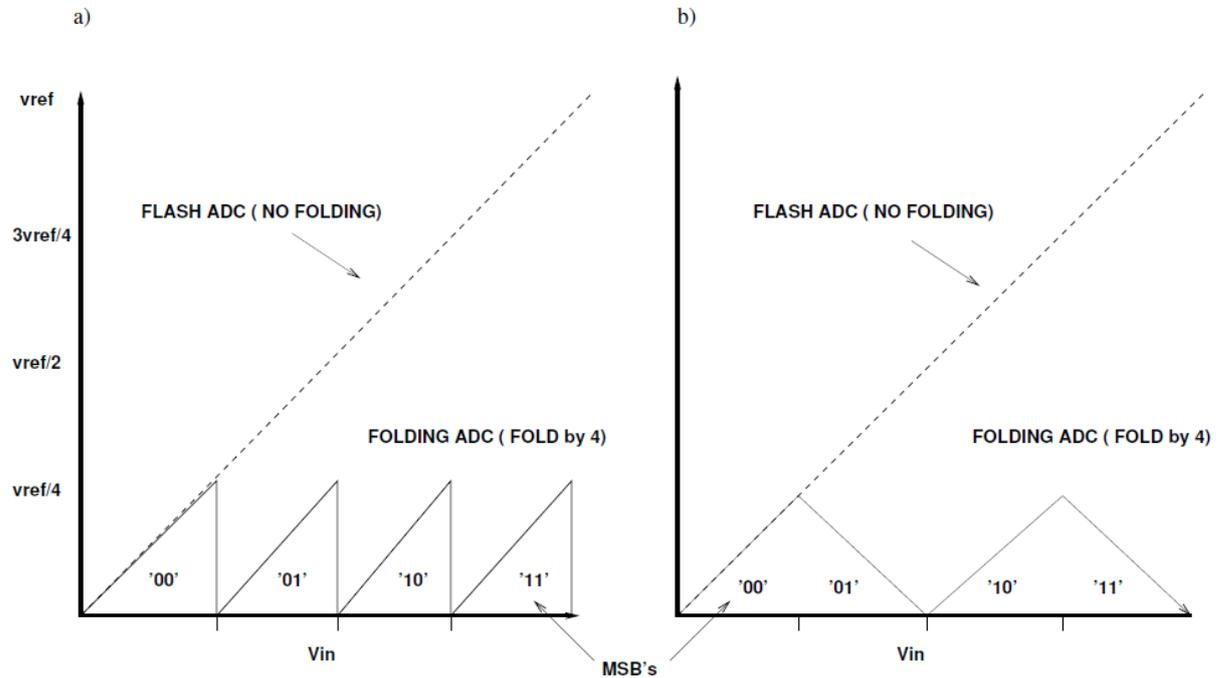
Fig. 2. a) Sawtooth characteristic b) Triangular characteristic
