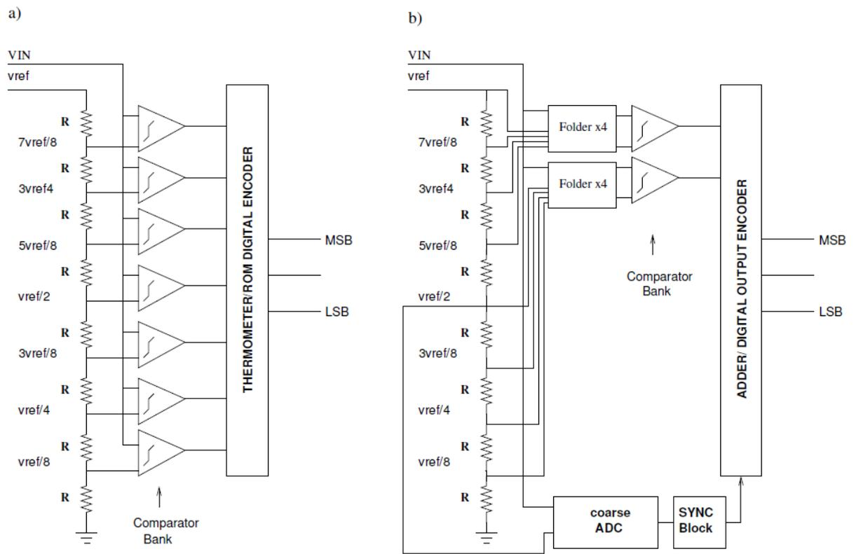
Fig. 1. Principle of folding.
